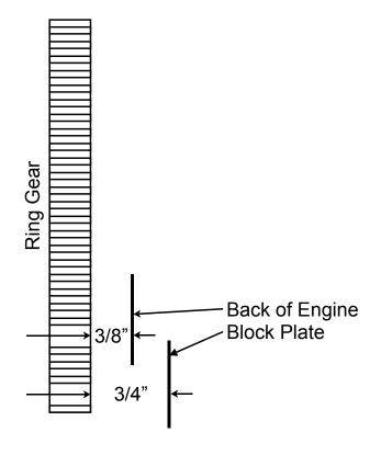
To determine exactly which Tuff Stuff starter to use, you need to take two measurements:
