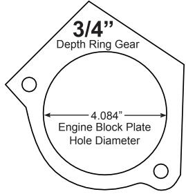
164 Tooth Ring Gear with Auto Trans or 157 Tooth Ring Gear with Auto or Manual Trans Use **3124**, **3149**, **6124**, **6585**, **6785**, **13124 or a 13149** Tuff Stuff starters
