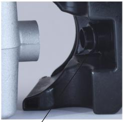
2. Install the O-ring on the reservoir outlet port. Lightly lubricate the O-ring with power steering fluid. Position reservoir on pump and hand press the two together.
