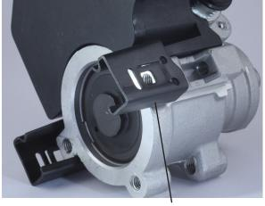
3. Note that there are two different clips and that each clip has a 90° edge that needs to be positioned against the pump and in the slotted groove. Partially install both retaining clips, wide end first.
