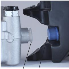
1. Remove port cover plugs from the pump inlet and the reservoir outlet.
