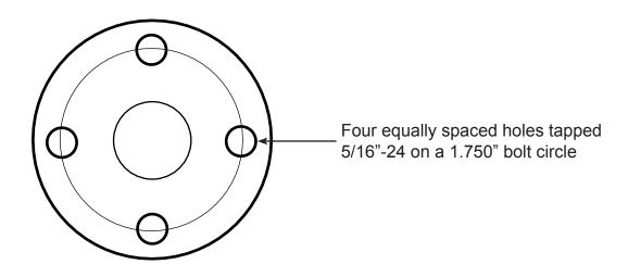
This hub is used on the 1594 and 1625 Ford water pump series
