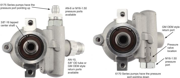
All Type II pumps have a 1200 PSI pressure and 3GPM flow rating. An optional 850PSI 2GPM valve is available separately.
