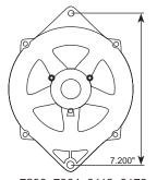
7290, 7864, 8112, 8173 Note that the top hole is not threaded on 7864 & 8112
