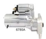
6785 has a 9-tooth pinion gear
