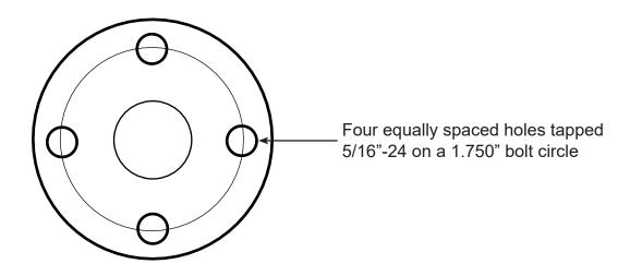
This hub is used on the 1594 and 1625 Ford water pump series
