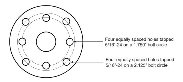
This hub is used on the following **Chevrolet** water pump series: 1493 and 1675
