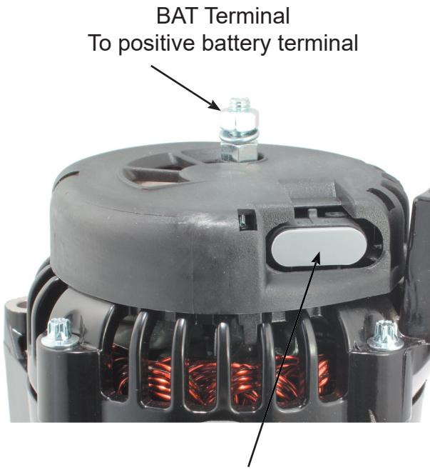
When using with OEM wiring harness, remove foam cover and plug in factory connector here
