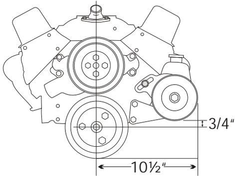
If the motor is to be equipped with A.C., The P.S. Pump should use a double groove pulley and the crankshaft a triple groove pulley. This will allow the use of a belt on the inner grooves of both the crankshaft and the power steering pump.
