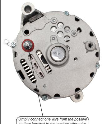
battery terminal to the positive alternator terminal. It's that easy!
