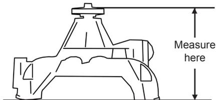
Measure from the top fan hub surface to the water pump mounting surface
